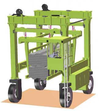
optional 6 wheels - reduces the wheel loading for use on poor quality pavements and docks with weight restrictions.
