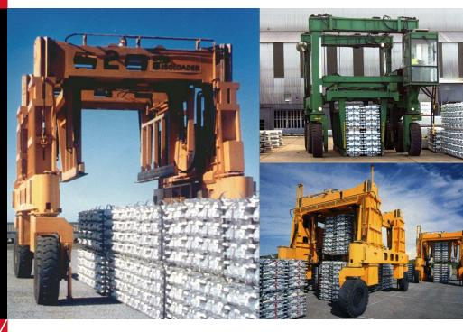
The Ingot Carrier can handle ingots bundles both at the smelter and at the port, and transport them in between at high speed.
